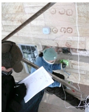
Electrochemical measurements were used to estimate how fast the rust was spreading. They showed little or no risk of corrosion on lower floors.
