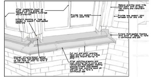
This building, now a luxurious condominium, was built in the 1920's using durable masonry construction. But it was plagued for decades by a patchwork of unexplained leaks, some worse than others. A \$1 million program of repairs, including pointing, was completed with very little effect. The condominium management looked for better advice and decided to call Leavitt Associates.
